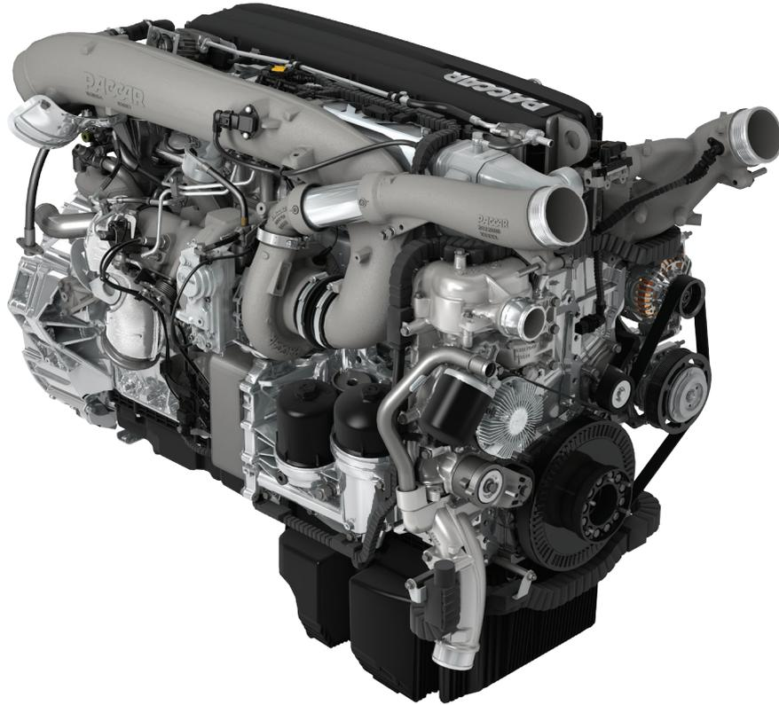
The 12.9 litre Euro 6 PACCAR MX-13 engine uses ultra-modern common rail technology, a turbo with variable geometry and advanced controls for maximum efficiency. In order to comply with the strict Euro 6 emissions requirements, it features exhaust gas recirculation, together with SCR technology and an active soot filter.
